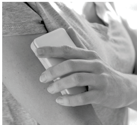
The Skulpt device (bottom) is marketed to consumers to take electrical impedance myography readings from muscles and record them through a smart phone app (top).
