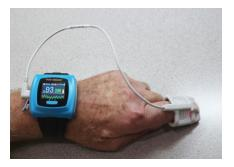
The device has the ability to store all the details overnight so that it can be connected to a computer the next day to analyze the data, issue a summary report and also a minute-by-minute graph of the heart rate and oxygen intake. The Pulse-Oximeter can also be attached for several minutes during the day to see current functions. There are specific guidelines for the minimum oxygen intake function for day and night.
